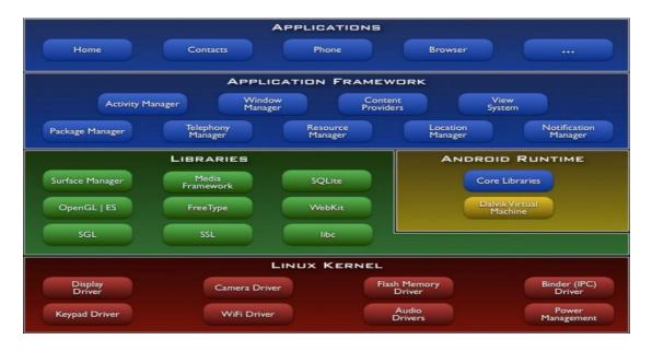
**Linux kernel:** This is the kernel on which Android is based. This layer contains all the low level device drivers for the various hardware components of an Android device.
