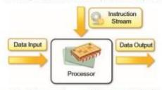
Single-instruction, multiple-data (SIMD) systems - An SIMD computing system is a multiprocessor machine capable of executing the same instruction on all the CPUs but operating on different data streams (see Figure 2.3). Machines based on an SIMD model are well suited to scientific computing since they involve lots of vector and matrix operations. For instance, statements such as Ci = Ai \* Bi
