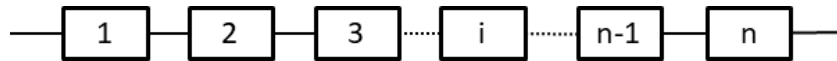
Fig. 1. A reliability block diagram depicting a series connection between a source and destination node pair.
