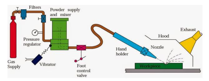
Construction of Abrasive Jet Machining (AJM):
