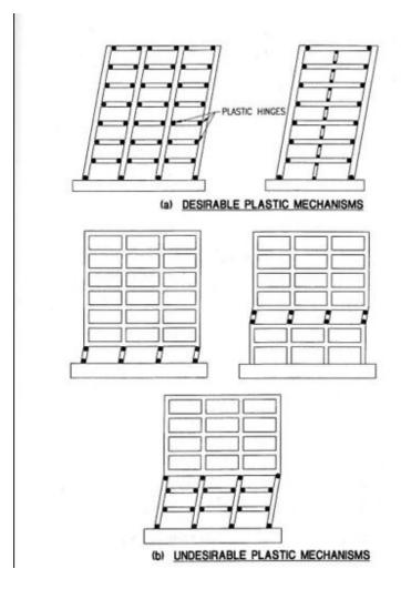
In building design we follow the philosophy of strong column and weak beam .that is so because in case of excessive load like in earthquake we want our beams to yield i. e., that is to fail but want our columns to be intact so that the whole structure stays even with some damage to beam so that the human cost can be minimized.
