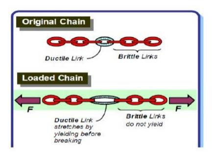
Comparing this concept to a lane frame, we want our structure to have ductile failure so
