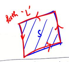
The Circulaturis of a rectus field if around a closed path L is equal to surface integral of curl of it ones the open surface s bounded by L, provided if & TXH are continuous on S.
