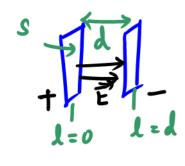
Capacitance of a parallel plate capacitor:
