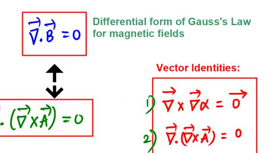
Comparing the above two equations, we can write Magnetic flux density in terms of vector potential
