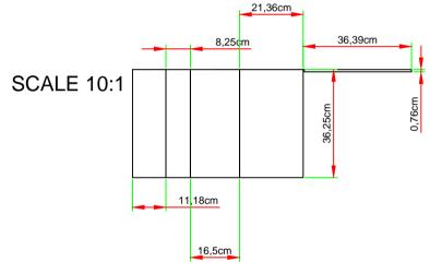
3 PHASE, CORE TYPE ,250KV,11KVV/400V TRANSFORMER SCALE 10:1 LV WINDING 43.5,HV WINDING 43.5 FRONT ELEVATION FULL IN SECTION AND PLAN IN FULL SECTION
