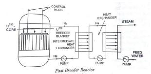
A fast breeder reactor is a small vessel in which the required quantity of **enriched uraniumor plutonium is kept** without a moderator.
