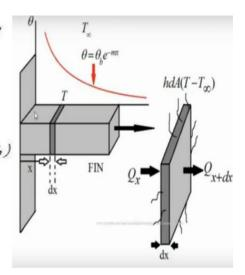
$\frac{d^{2}T}{dx^{2}} - \frac{hP}{KA_{c}}(T - \overline{b}_{0}) = 0$   $Taking \frac{hP}{KA_{c}} = m^{2} \text{ and } T - \overline{b}_{0} = 0 \Rightarrow \frac{\partial^{2}\theta}{\partial x^{2}} = \frac{\partial^{2}T}{\partial x^{2}} \Rightarrow \frac{d^{2}\theta}{dx^{2}} = \frac{d^{2}T}{dx^{2}}$
