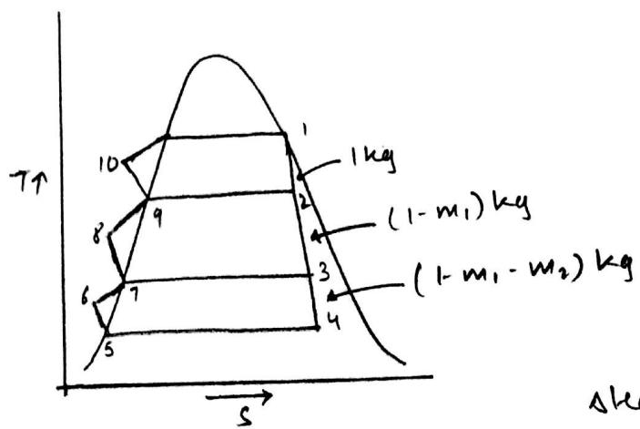
In a practical regenerative cycle the feed water enters the boiler. The temp between 10 and 40 and it is heated by a stream excited by a boiler. The flow diagram of the regenerative cycle with saturated steam at the inlet of the turbine
