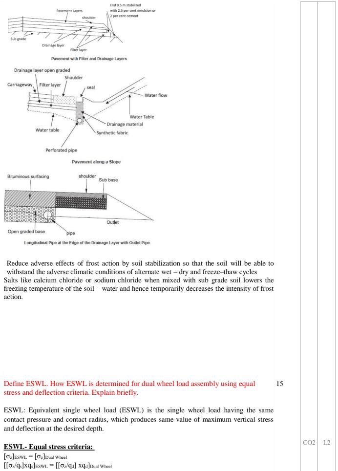
$\begin{bmatrix} [\sigma_z/q_s] X q_s]_{ESWL} = \begin{bmatrix} [\sigma_z/q_d] X q_d]_{Dual Wheel} \\ Since the area remains same \\ \begin{bmatrix} [\sigma_z/q_s] X P_s]_{ESWL} = \begin{bmatrix} [\sigma_z/q_d] X P_d]_{Dual Wheel} \\ P_s/P_d = [\sigma_z/q_d] / [\sigma_z/q_s] \end{bmatrix}$
