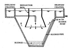
a. The maximum daily demand at a water purification plant has been estimated as 12 million litres per day. Design the dimensions of a suitable sedimentation tank (Fitted with mechanical sludge removal arrangements) for the raw supplies, assuming a detention period of 6 hours and velocity of flow as 20cm/min. (06 Marks)
