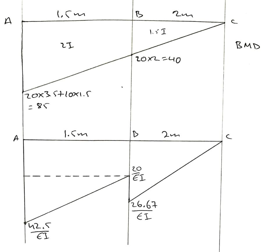
$$(1) \text{ Slope at } C \Rightarrow \theta_c = \frac{1}{2}(2)\left(\frac{26.67}{EI}\right) + \left(1.5 \times \frac{20}{EI}\right) + \left(\frac{1}{2}(1.5)\left(\frac{42.5}{EI}\right)\right)$$
