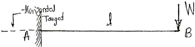
Z(a) Calculate the slope and deflection at free end by using moment area method.
