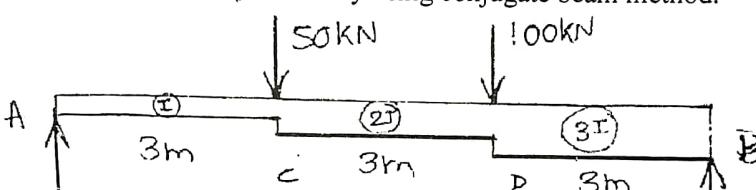
Z(a) Determine the slope and deflection at free end by using conjugate beam method.
