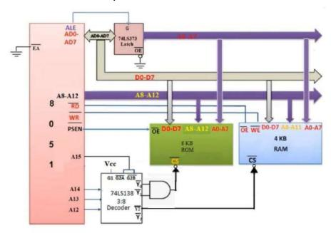
Interface 4k bytes of RAM and 8k bytes ROM to 8051 microcontrollers in such a way that starting address of RAM is C000H and ROM is 0000H.
