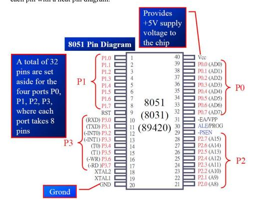
Pins 1-8 (PORT 1). It has 8 pins It can be used as input or output. It already has internal pull-up resistors. Hence no external pull-up resistors are required. On Reset port1 is configured as I/P port by writing 1 to all its bits.
