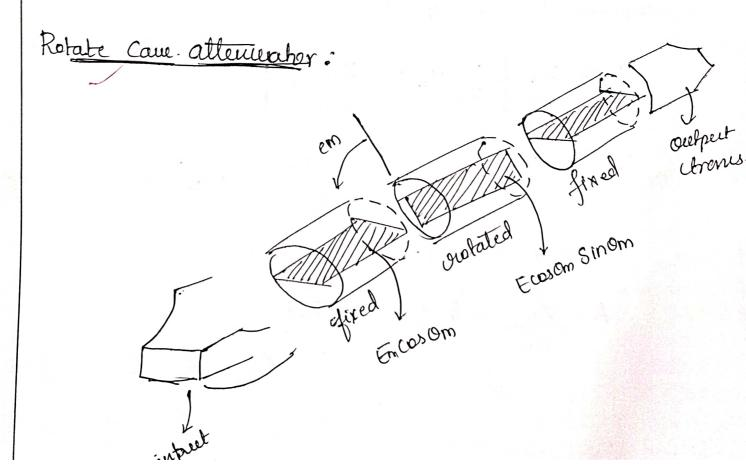
There are three main successive parts two fixed and one violated There are two steenhams input itrans and the output trans where there will less SWR. Attituation can be controlled by violating.
