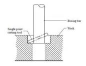
**Countersinking** - It is the operation of making a cone-shaped enlargement of the end of hole to provide a recess for a flat head screw or countersunk rivet fitted into the hole. The tool used for countersinking is called a countersink. Standard countersunks have  $60^{\circ}$ ,  $82^{\circ}$  or  $90^{\circ}$  included angle and the cutting edges of the tool are formed at the conical surface. The cutting speed in countersinking is 25% less than that of drill.
