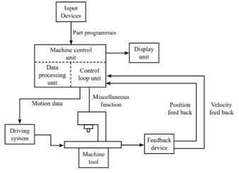
The machine control unit (MCU) is a microcomputer
