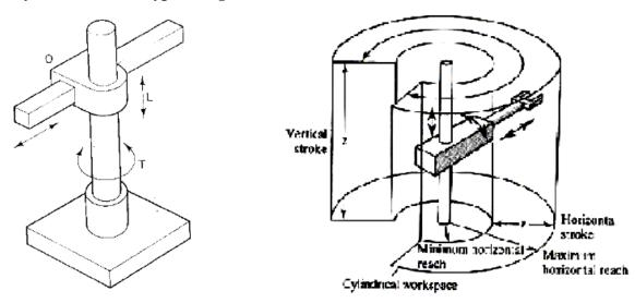
Notation: [TLO]: Twisting, Linear and Orthogonal
