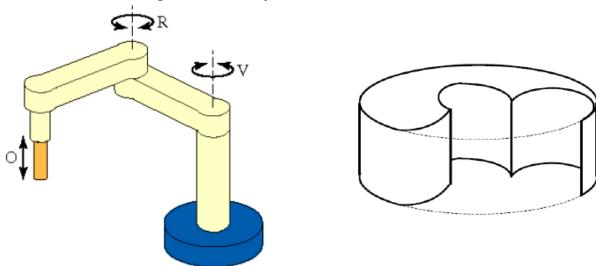
Notation: [VRO]: Revolving, Rotational and Orthogonal joint
