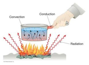
**Radiation** - It is the process in which heat is transferred from one body to another body without involving the molecules of the medium. Radiation heat transfer does not depend on the medium.
