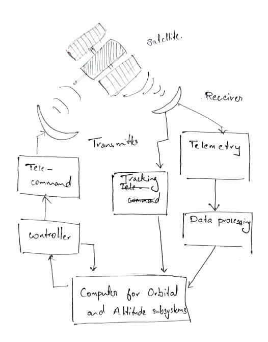
The telemetry, tele command of Tracking control
