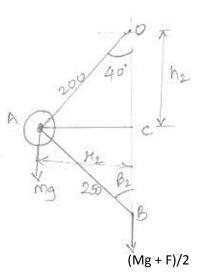
Given: - OA = 200 mm = 0.2m; AB = 0.25m, M = 15 kg, m = 2 kg; F = 24N; \( \pi\_1 = 30^\circ, \pi\_2 = 40^\circ
