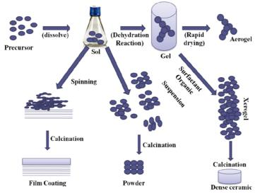
Step1: Formation of different stable solutions of the alkoxide or solvated metal precursor (the sol).
