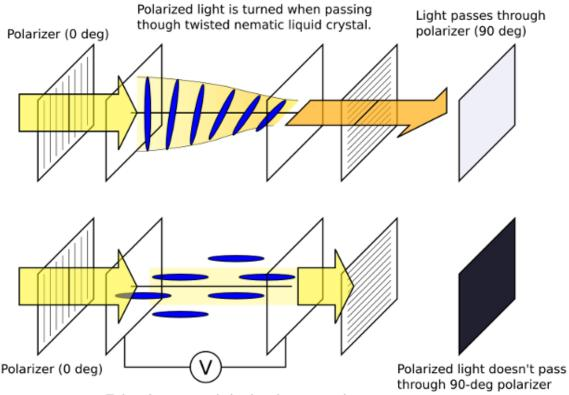
Twisted structure is broken by external electric filed. Polarized light is not turned.
