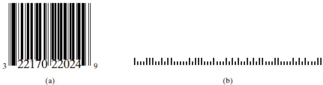
Figure 12.1 Two forms of linear bar codes are (a) width-modulated, exemplified here by the Universal Product Code, and (b) height-modulated, exemplified here by Postnet, used by the U.S. Postal Service.
