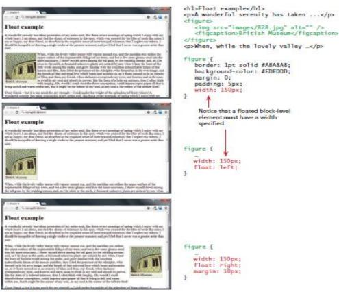
FIGURE 5.9 Floating an element
