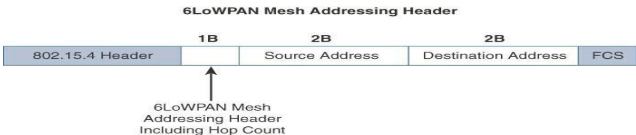
Figure 3.6 6LoWPAN Mesh Addressing Header
