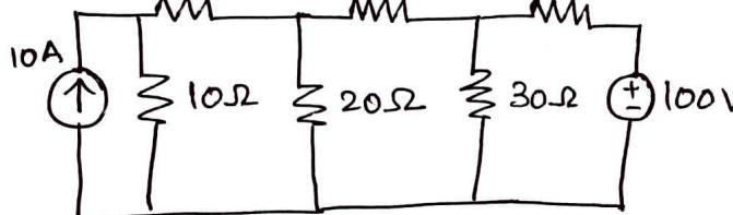
Converting current source to voltage source and then  $10\Omega$  is in series with
