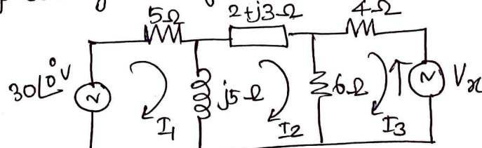
Applying KVL to mesh I<sub>1</sub>,
