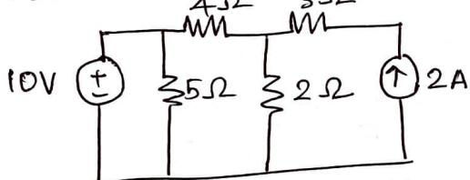
Considering a single voltage source of 10V and the current source is kept open. So the 4Ω and 2Ω resistors are connected in series, which is parallel with 5Ω resistor.
