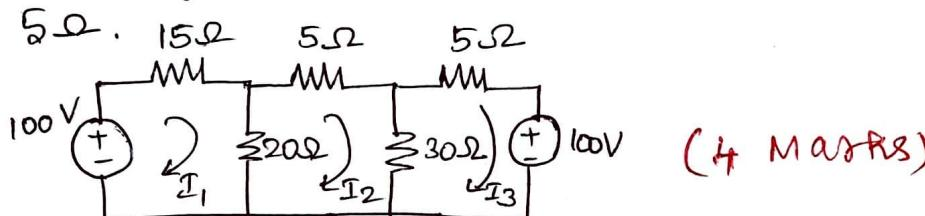
Applying the KVL for the loop
