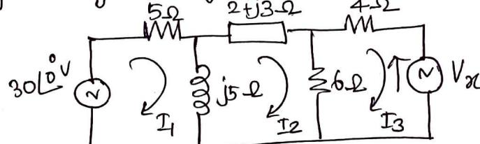
Applying KVL to mesh I<sub>1</sub>,
