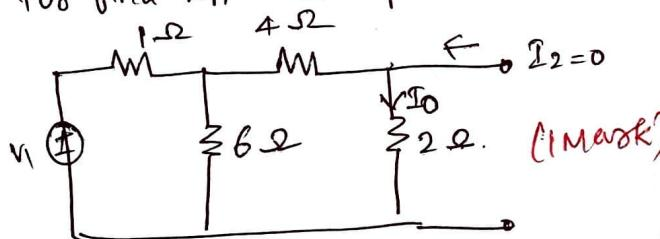
$$Z_{11} = \frac{V_1}{I_1} \Rightarrow \text{Resistance } R = \frac{6 \times 4}{6+4} + 1 = 4 \Omega$$
