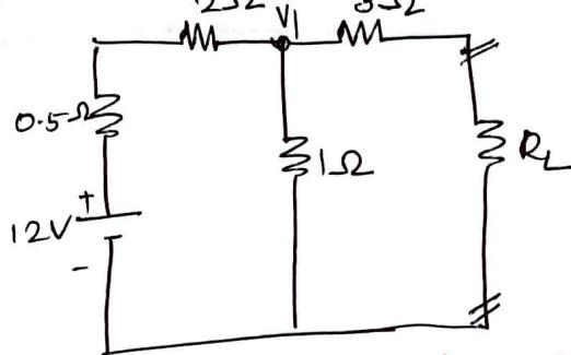
$$V_{TH} = V_1$$
