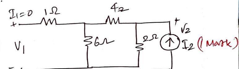
$$Z_{22} = \frac{V_2}{I_2} = 2 \times (4+6) = 20 \Omega$$
