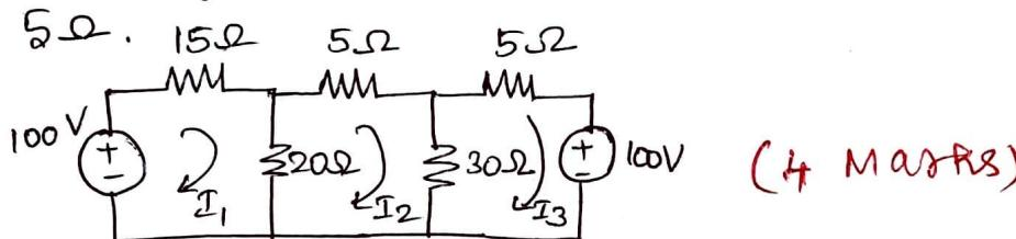
Applying the KVL for the loop
