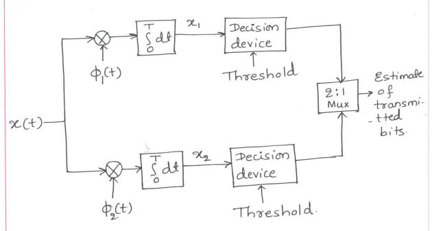
Let x(t),  $0 \le t \le T$  be the received symbol.  $x(t) = S_i(t) + \omega(t)$ ,  $0 \le t \le T$  i = 1, 2, 3, 4
