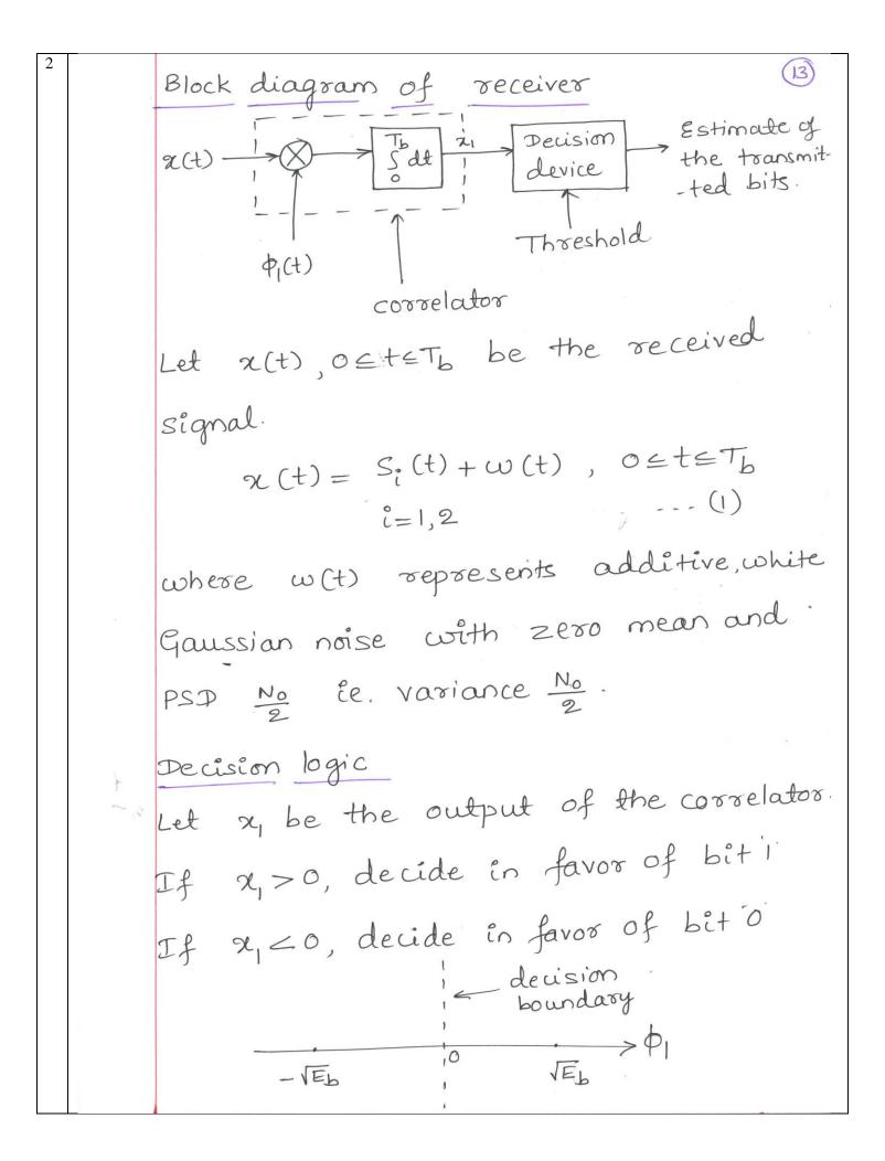
Suppose that bit is was transmitted. ce, s<sub>2</sub>(t) was transmitted.
