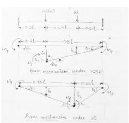
from beam mechanism under load  $\omega$ .  $S_{2=0.75} \downarrow \theta_1 = 0.25 \downarrow \theta_2 \qquad \text{(iv)}.$   $\theta_{2=0.75} \downarrow \theta_1 \qquad 0.25 \downarrow \text{(iv)}.$   $0.25 \downarrow \downarrow 0.25 \downarrow \text{(iv)}.$
