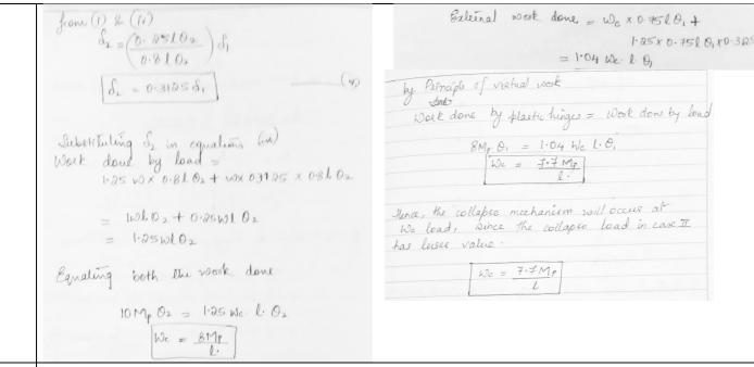
5 Find required value of plastic moment capacity of the continuous beam as shown in figure 3. The loads shown are collapse loads.
