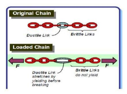
Comparing this concept to a lane frame, we want our structure to have ductile failure so that the structure would be able to take large deformations in its inelastic zone. For this to be applicable, we need to make one structural element to behave relatively ductile to the others. We chose beams to behave relatively ductile compared to columns. (If we chose columns to be ductile then whole building would collapse as shown).
