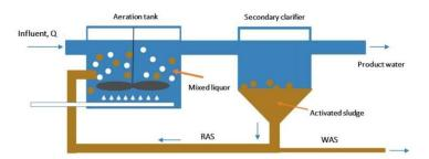
**Extended Aeration Activated Sludge** - The extended aeration activated sludge process operates in the endigenous respiration phase of the growth curve, which necessitates a relatively low organic loading (low F/M) and long aeration time.
