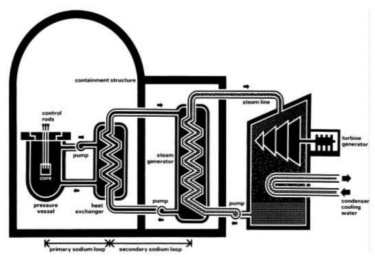
The breeder-reactor design concept is predicated on maximizing new fuel production in breeding more fuel than used to sustain the neutron chain reaction. For this purpose, fissile plutonium and fertile <sup>238</sup>U fuel with fast neutrons have been found to be the most efficient.
