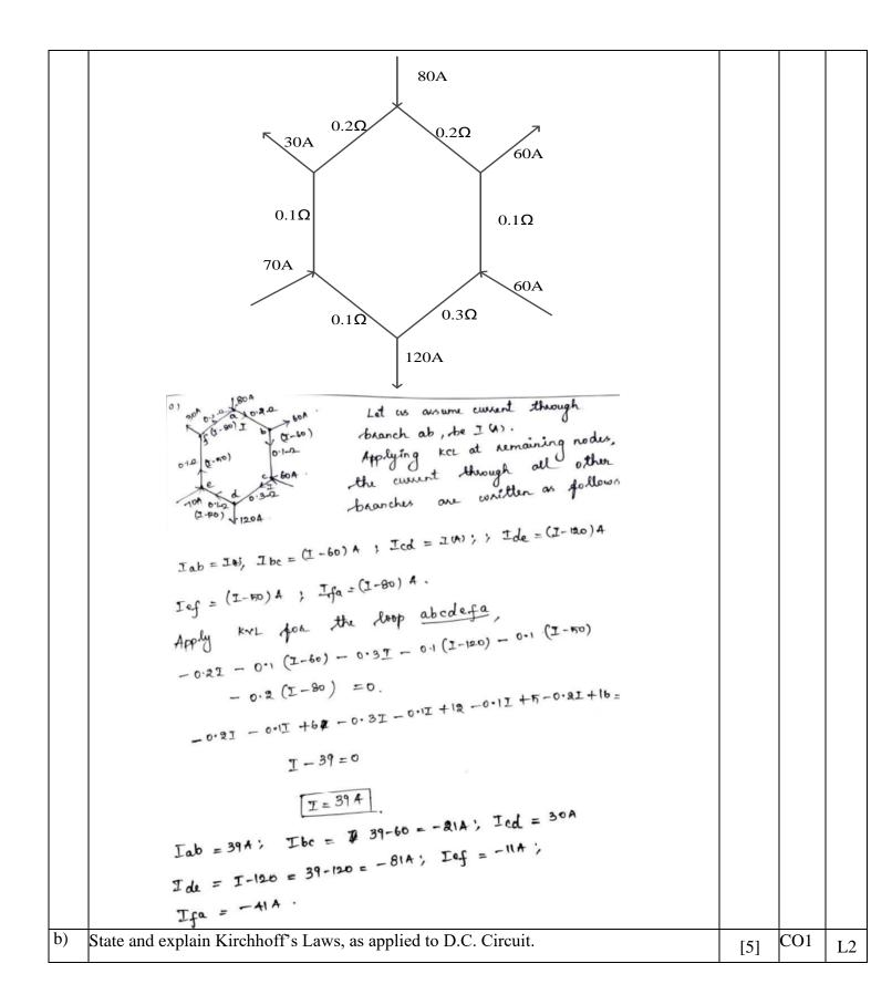
The current or voltage of any circuit branch can also be calculated using Kirchhoff's Law. These laws are valid in AC and DC networks at low frequencies.
