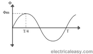
As, shown in the fig., the flux rises sinusoidally to its maximum value  $\Phi m$  from 0. It reaches to the maximum value in one quarter of the cycle i.e in T/4 sec (where, T is time period of the sin wave of the supply = 1/f).
