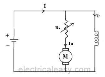
**Speed of a dc motor** is directly proportional to the back emf  $E_b$  and  $E_b = V - I_a R_a$ . That means, when supply voltage V and the armature resistance  $R_a$  are kept constant, then the speed is directly proportional to armature current  $I_a$ . Thus, if we add resistance in series with the armature,  $I_a$  decreases and, hence, the speed also decreases. Greater the resistance in series with the armature, greater the decrease in speed.
