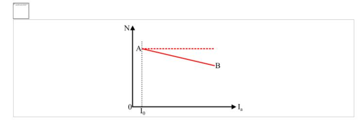
For a DC shunt motor, the back EMF and flux both are constant under normal operating conditions. Therefore, the speed of a shunt motor will remain constant with respect to armature current as shown by dotted line.
