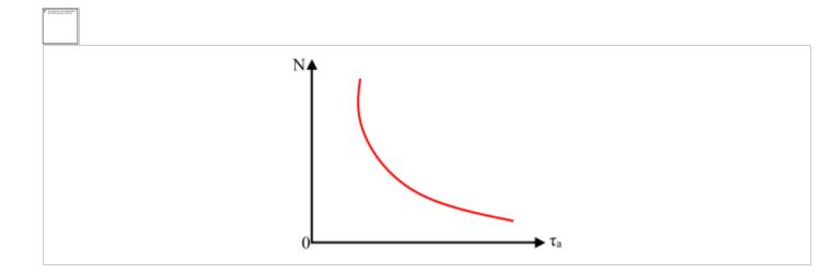
It is clear from the characteristics that the series motor has high torque at low speed and vice-versa. Thus, the series DC motor is used where high starting torque is required.
