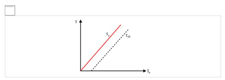
Hence, the torque and armature current characteristics of DC shunt motor is straight line passing through the origin (see the figure). The shaft torque is less than the armature torque which is represented by the dotted line.
