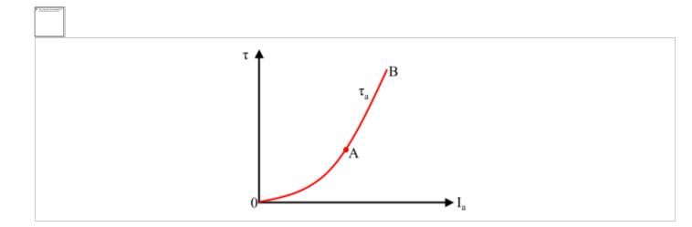
Therefore, up to magnetic saturation, the armature torque is directly proportional to the square of the armature current. Hence, the torque versus armature current curve upto magnetic saturation is a parabola (part OA of the curve).
