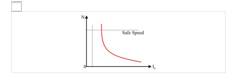
Hence, up to magnetic saturation the speed versus armature current curve is a hyperbola while after the magnetic saturation, the flux becomes constant and hence the speed
