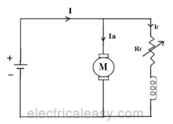
It is already explained above that the **speed of a dc motor** is inversely proportional to the flux per pole. Thus by decreasing the flux, speed can be increased and vice versa.
