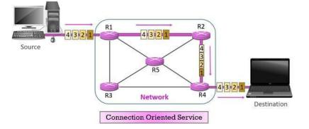
To establish a connection a source sends a **request** packet to the destination. In response to which destination sends the **acknowledgement** packet to the source confirming that the destination is ready to accept the data from the source.
