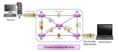
Each datagram carries its **source** and **destination** address. The **router** uses the **destination** address to route the datagram to its destination. The packets received at the destination may be received **out of order**. Hence, the datagrams are assembled to recreate the original message. The **UDP** protocol is a **connectionless** protocol.
