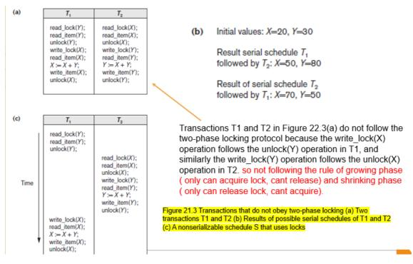
□ If we enforce two-phase locking, the transactions can be rewritten as T1' and T2' as shown in Figure 22.4.
