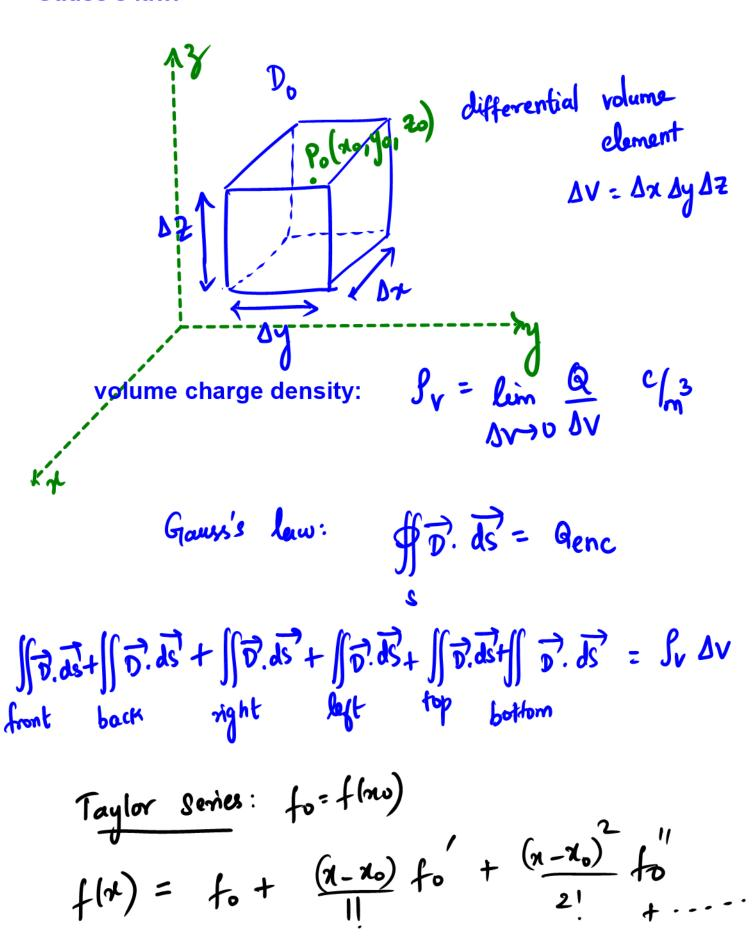
$$\iint_{\text{front}} + \iint_{\text{back}} \vec{D} \cdot \vec{ds} = \frac{\partial D_x}{\partial x} \Delta x \Delta y \Delta z$$
