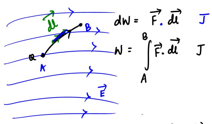
Force on the point charge in the electric field,  $\overrightarrow{F} : Q \overrightarrow{E}$
