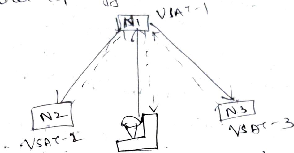
As the name suggests it is bidirectional, that means it can send and receive the data at the same time. It is like dual two way communication.
