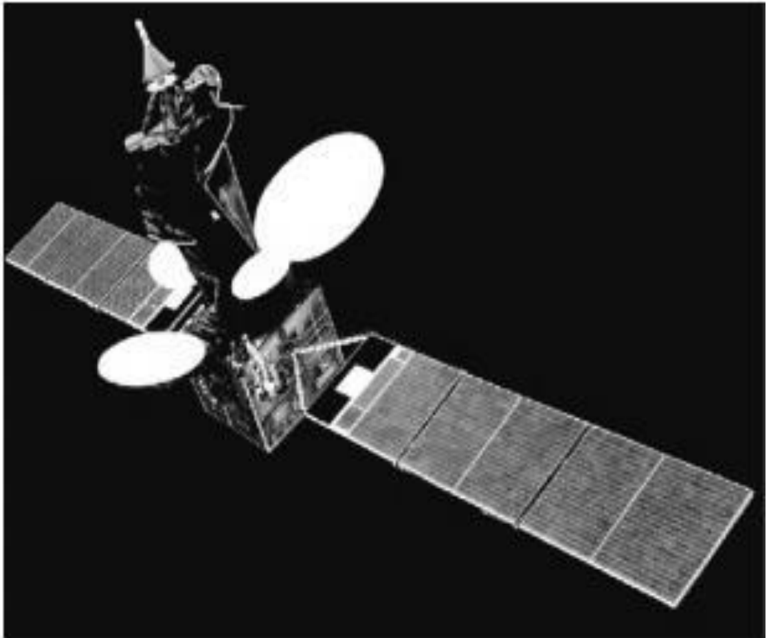
Fig: Three-axis stabilized satellite (Intelsat-5) (Reproduced by permission of © Intelsat)
