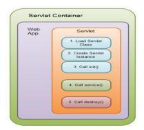
The servlet is initialized by calling the init () method.
