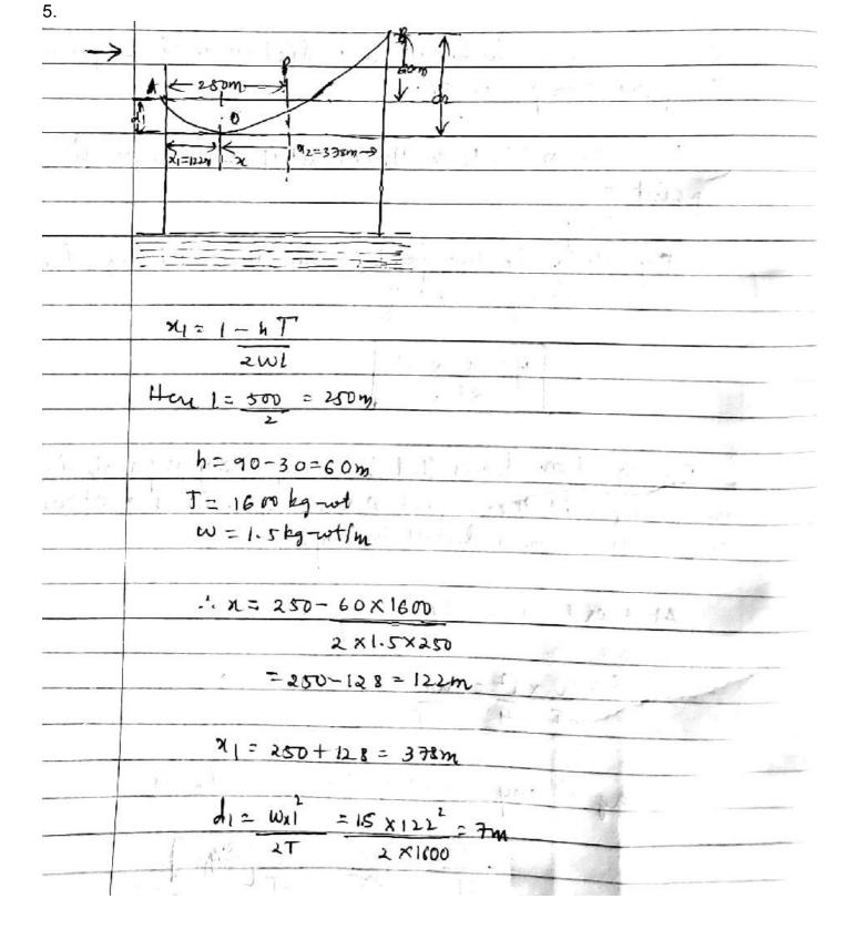
As seen from fig, clearance of the lowest poort o for = 30-7=23m The Horizontal distance of mid-point p from the reference point 0 is n = (250 - 122) = 128m. The height of the point P above 0 is divid = Wx12 = 1.5×1282 = 7.68 m 21 2×1600 Hence, clearance of mid-pant above water level 23+7.68=30,68m
