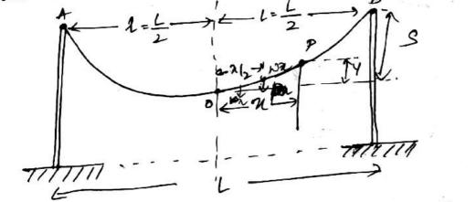
The point & is the breat point on the trajectory. O is the midspan as shown aifig. L = lengte of span cimetees N = weight open mit lengte of landweber in 1/m T T = Tension in the conductor in kg
