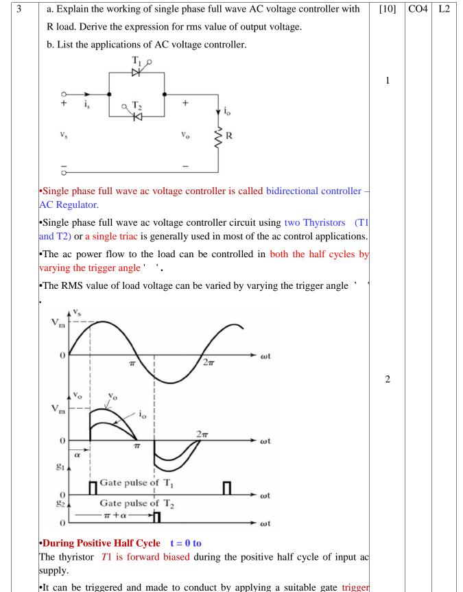
pulse ' '. only during the positive half cycle of input supply.
