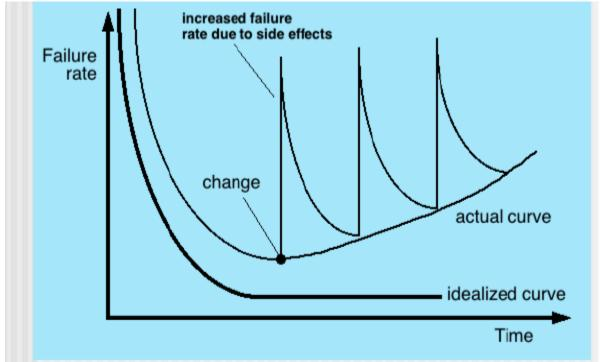
Before the curve can return to the original steady-state failure rate, another change is requested, causing the curve to spike again. Slowly, the minimum failure rate level begins to rise—the software is deteriorating due to change.When a hardware component wears out, it is replaced by a spare part. There are no software spare parts. Every software failure indicates an error in design or in the process through which design was translated into machine executable code.
