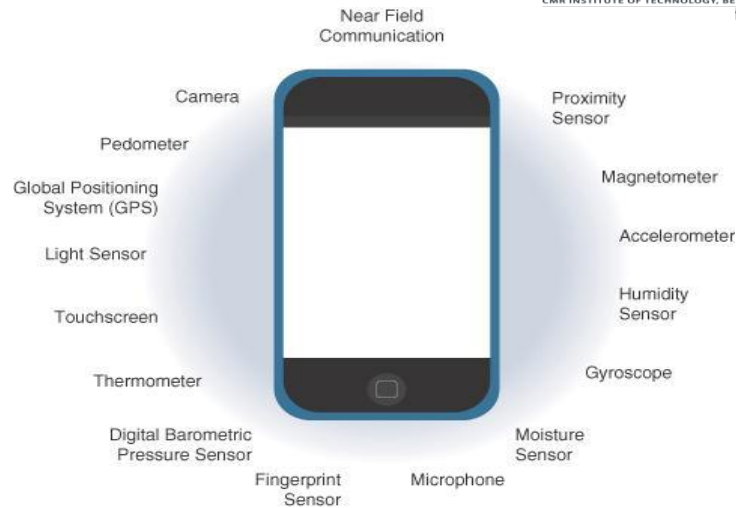
Figure 2.1: Sensors in a smart phone
