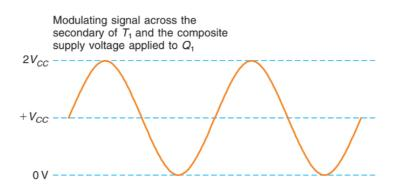
A major disadvantage of collector modulators is the need for a modulation transformer that connects the audio amplifier to the class C amplifier in the transmitter. The higher the power, the larger and more expensive the transformer. for 100 percent modulation, the power supplied by the modulator must be one-half the total class C amplifier input power.
