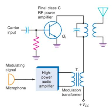
With a zero-modulation input signal, there is zero-modulation voltage across the secondary of T1, the collector supply voltage is applied directly to the class C-amplifier, and the output carrier is a steady sine wave.
