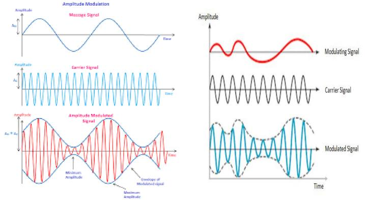
Frequency Domain Representation: (2M+2M)To arrive at frequency domain representation, take the Fourier transform of s(t)  $S(f) = \int_{-\infty}^{\infty} s(t)e^{-j2\pi ft} dt$   $S(f) = F(V_c [1 + k_a m(t)]Sin (2\pi f_c t))$   $S(f) = F[A_c Sin (2\pi f_c t)] + F[A_c k_a m(t)Sin (2\pi f_c t)] -----(1)$ Note: magnitude spectrum is considered
