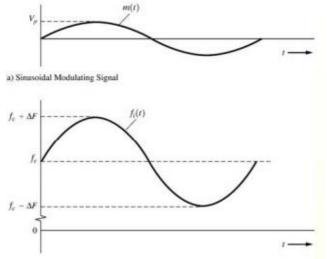
Modulation Index: It shows the depth of modulation. This is the ratio of deviation and bandwidth of the message signal (2M). The bandwidth of FM is majorly defined by beta. Beta= $(kf^*Vm)/fm$
