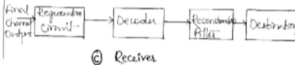
Fig(6) : The basic elements of a PCM system.
