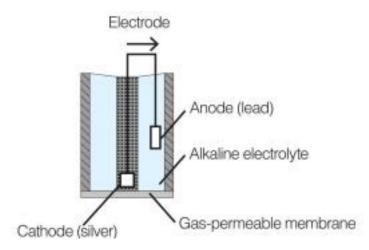
When the Clark electrode is immersed in a liquid sample, oxygen molecules diffuse through the hydrophobic layer and react with the cathode surface, producing a current that is proportional to the amount of oxygen present in the water.
