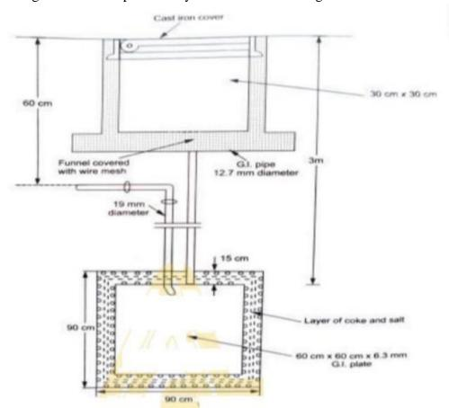
The earthing efficiency increases with the increase of the plate area and depth of the pit. The depth of the pit depends upon the resistivity of the soil. The only disadvantage of this method is that discontinuity of earth wires from the earthing plate which is placed below the ground as it cannot be observed physically this may cause miss leading and result into heavy losses under fault condition.
