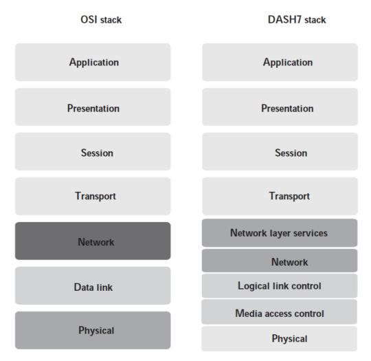
DASH7 stack includes support for cheap processing systems by virtue of its integrated file system. Figure 7.15 shows the protocol stack of DASH 7 in comparison to the ISOOSI stack. DASH7 gateways can query devices in proximity to it without waiting for pre-defined time-slots to listen to end-device beacons.
