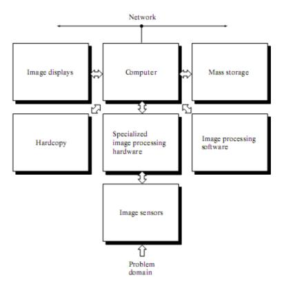
Although large-scale image processing systems still are being sold for massive imaging applications, such as processing of satellite images, the trend continues toward miniaturizing and blending of general-purpose small computers with specialized image processing hardware. Figure 3 shows the basic components comprising a typical general-purpose system used for digital image processing. The function of each component is discussed in the following paragraphs, starting with image sensing.
