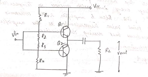
> Due to the existence of voltage devides cheevit a each transiste is braised by around 0.60 making Icea home the ideal value, Ict = 0.
